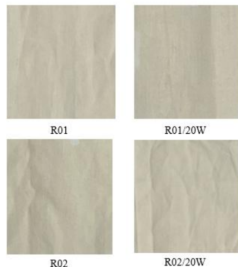
Figure 8. Fabric images of R01 and R02 without washing and with 20 repeated washings(20W)
