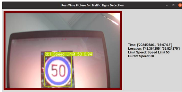
Figure 10. Real-Time test image of the accelerated model with TensorRT.
