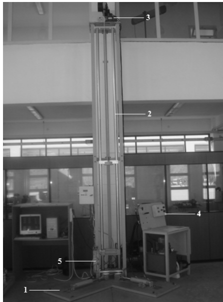
Figure 1. Drop-weight test machine: 1) L-shaped base steel plate, 2) drop weight tower, 3) elevator, 4) control unit, 5) brake system.
