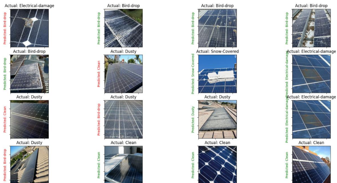
Figure 3. Visuals of some of the factors that cause failure ( https://www.kaggle.com/code/madenenivamsikrishna/fault-detection )
