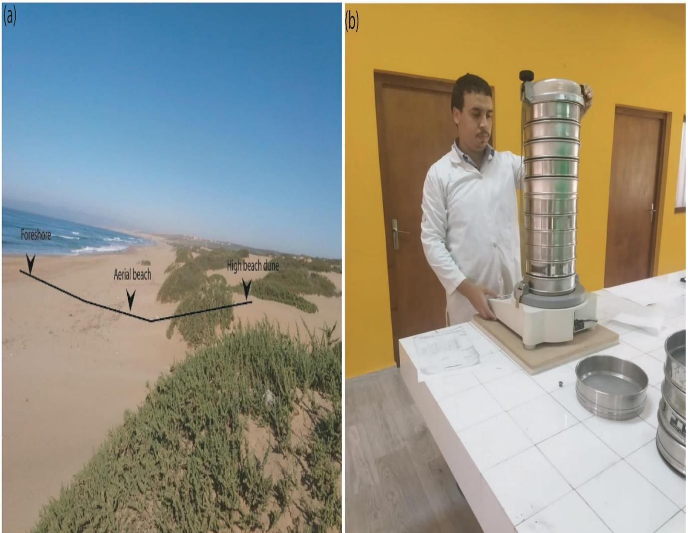
**Figure 5.** (a) Morphological units sampled on the Massa beaches, (b) Laboratory work: sieving using an AFNOR-type sieve.
