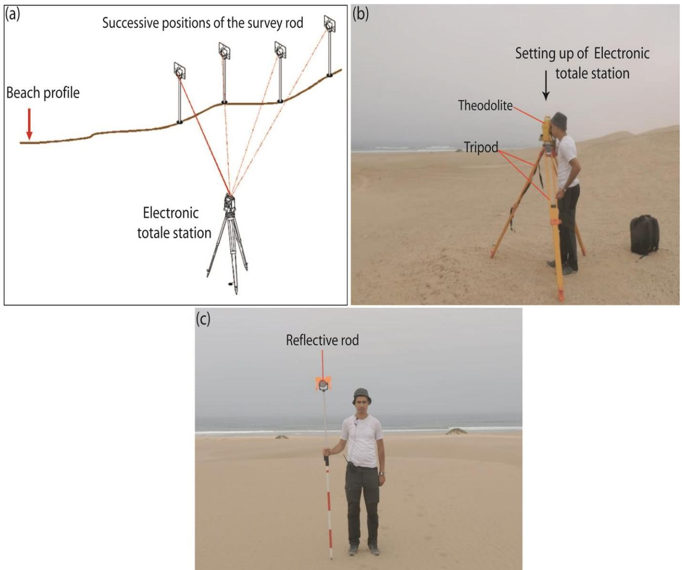
**Figure 3.** Measurement instrument used for topographic surveys, (a) Principle of beach profile surveys, (b) Setting up the SOUTH NTS-375R total station, (c) The reflective target.
