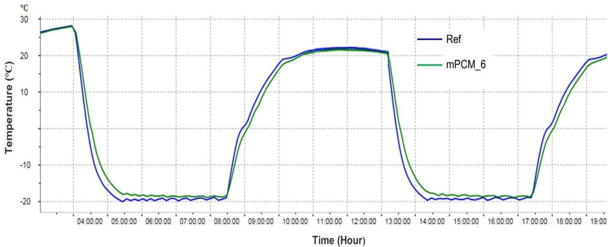
Figure 10. Internal Temperatures of Mortars After The Freezing-Thawing Cycle
