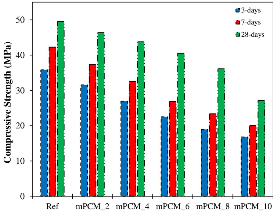
Figure 4. Compressive Strength Results
