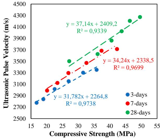
Figure 9. Relationship Between Compressive Strength – UPV
