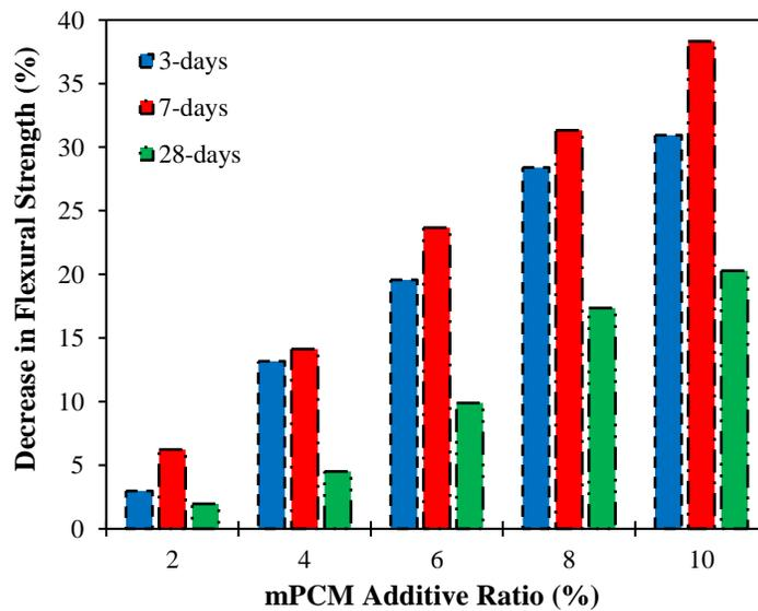
Figure 3. Percentage Decrease Rates In Flexural Strengths
