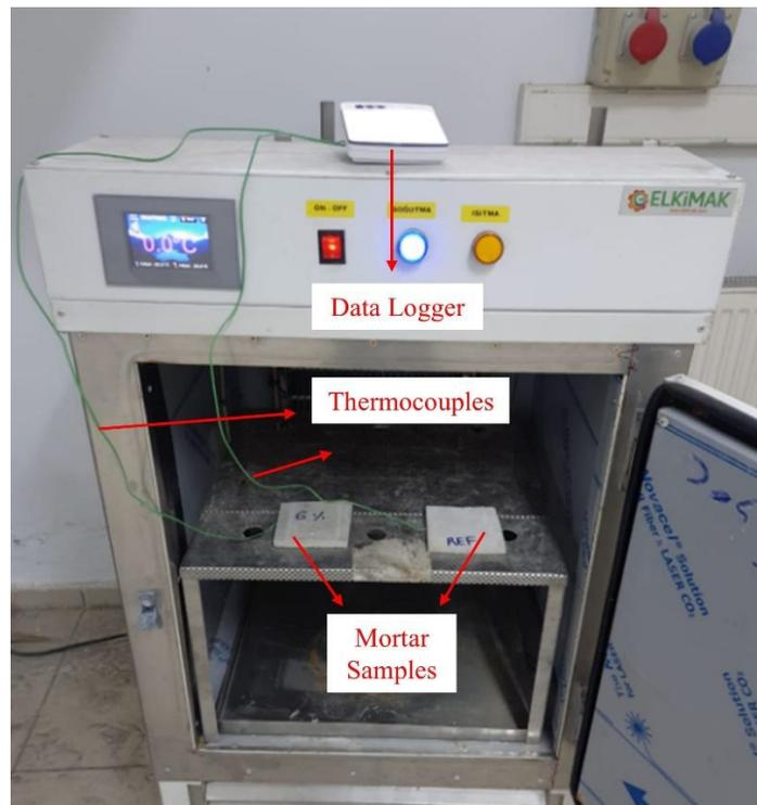
**Figure 1.** Experimental Setup Used To Monitor The Internal Temperature Changes of Mortars
