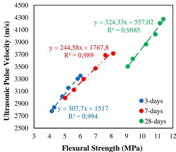
**Figure 8.** Relationship Between Flexural Strength – *UPV*
