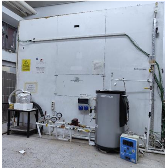
Figure 5. View of the radiator test measurement set-up
