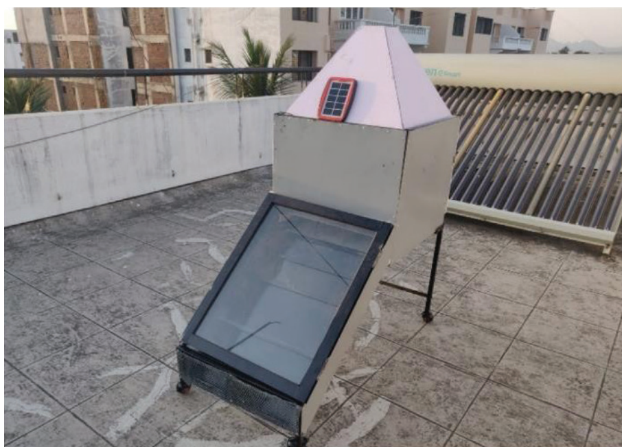
Figure 3. Indirect cabinet solar dryer [From Kokate et al. [59], with permission from Elsevier].
