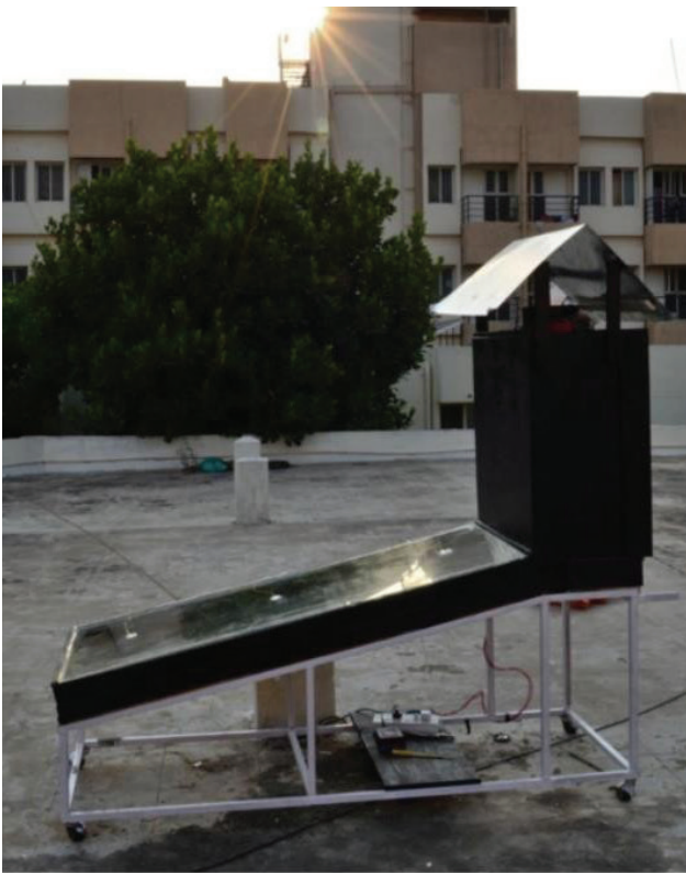
Figure 21. Indirect active solar dryer [From Hegde et al. [76], Open access].
