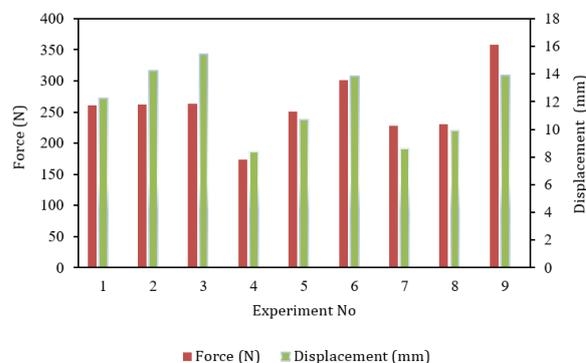
Figure 7. Force-displacement values of L-joint samples.
