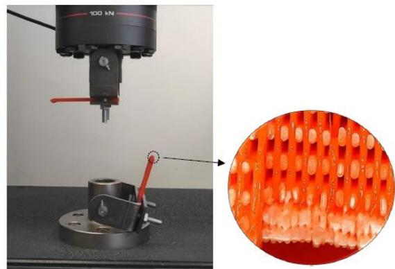
Figure 4. The tensile test applied to L-joint element.
