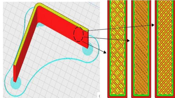
Figure 5. Grid (a), zigzag (b) and line (c) pattern.
