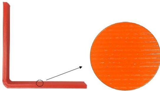
Figure 2. The l-joint sample produced with a 3D printer.
