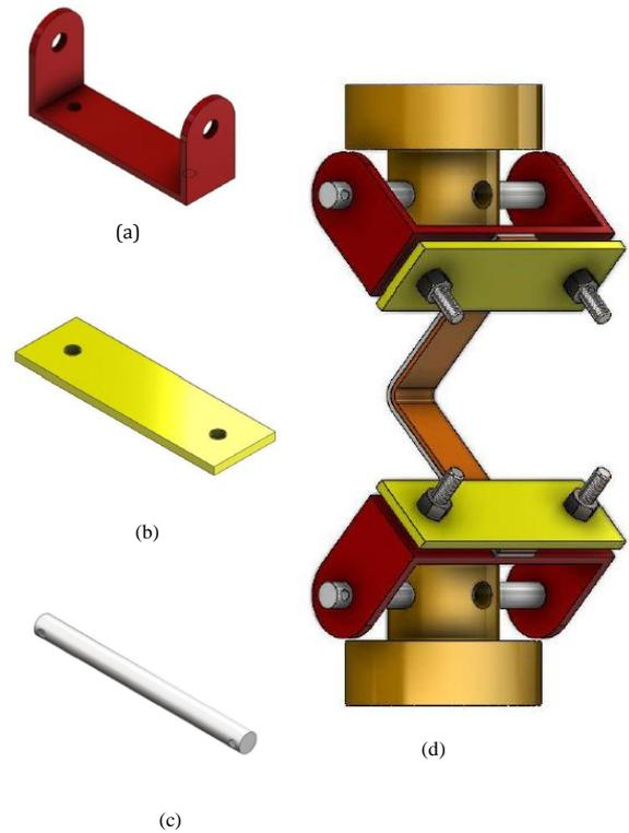
Figure 3. The jaw (a), bottom plate (b), pin (c) and assembly drawing (d).
