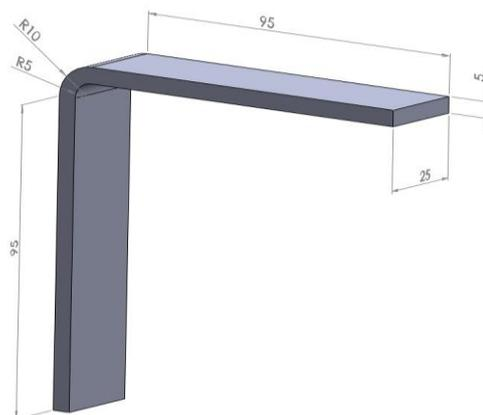
**Figure 1.** L-joint sample dimensions.
