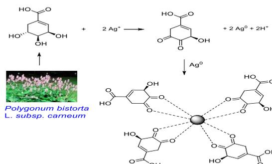
**Figure 2.** The reaction mechanism of synthesis of AgNPs.
