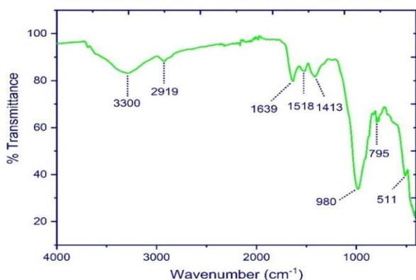
Figure 3. FTIR spectrum of nanostructure.
