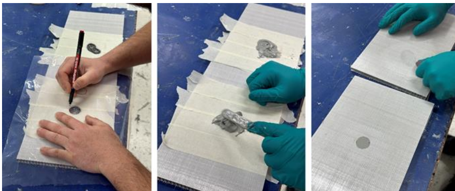
Fig. 7. Template creation, filler material application, and shaving process.
