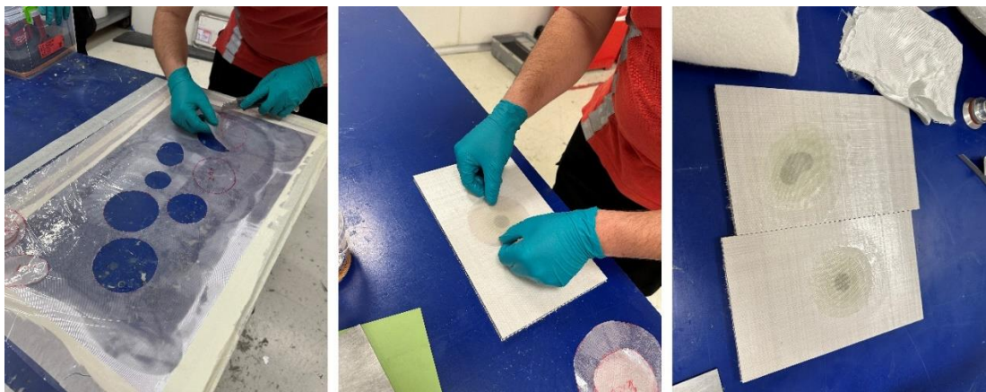
Fig. 9. Removal of fabric templates and fabric laying process.
