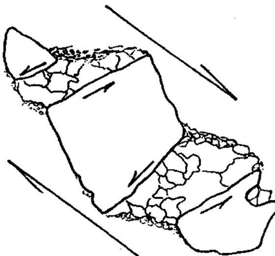
**Fig.5– Sketch showing sense and direction of movements of rotated clasts.**
