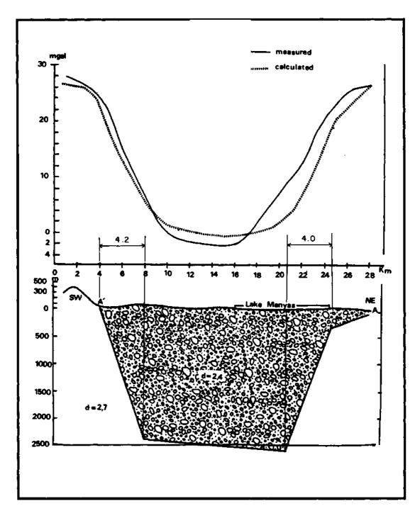
Fig. 2- The separation in the Bursa-Gönen graben, deduced from a gravimetric model.
