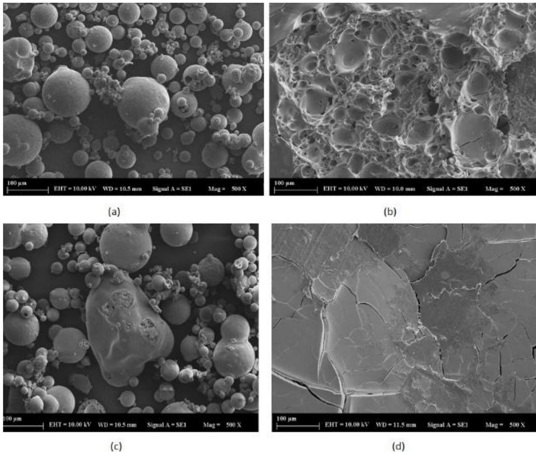
**Figure 5:** SEM images of tablets (a) T1 powder form before pressing, (b) T1 tablet form, (c) T5 powder form before pressing, (d) T5 tablet form.
