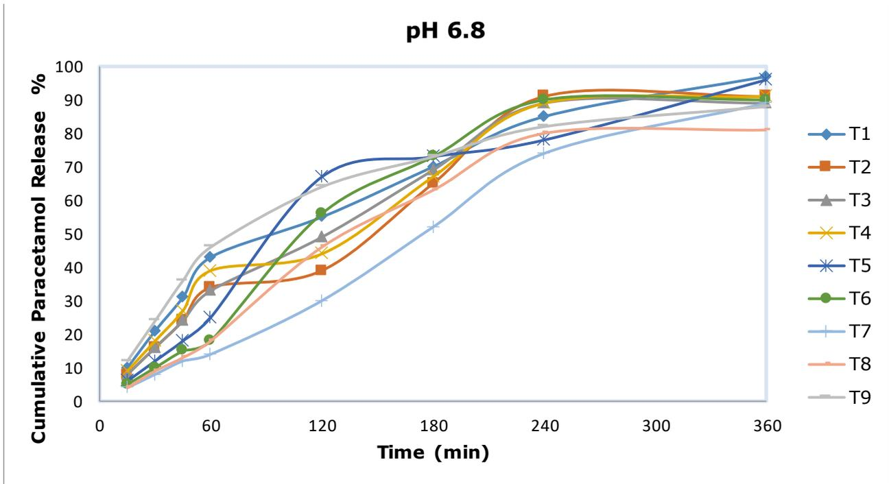
Figure 7: Paracetamol release profiles of matrix tablets at pH 6.8.
