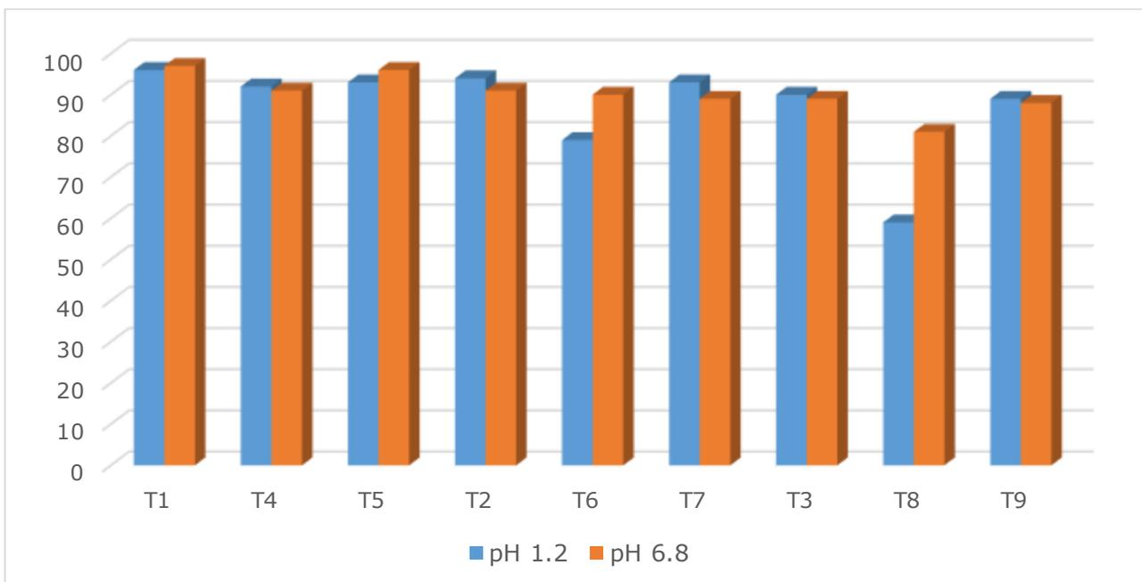
Figure 8: Paracetamol maximum release profiles at pH 1.2 and pH 6.8.
