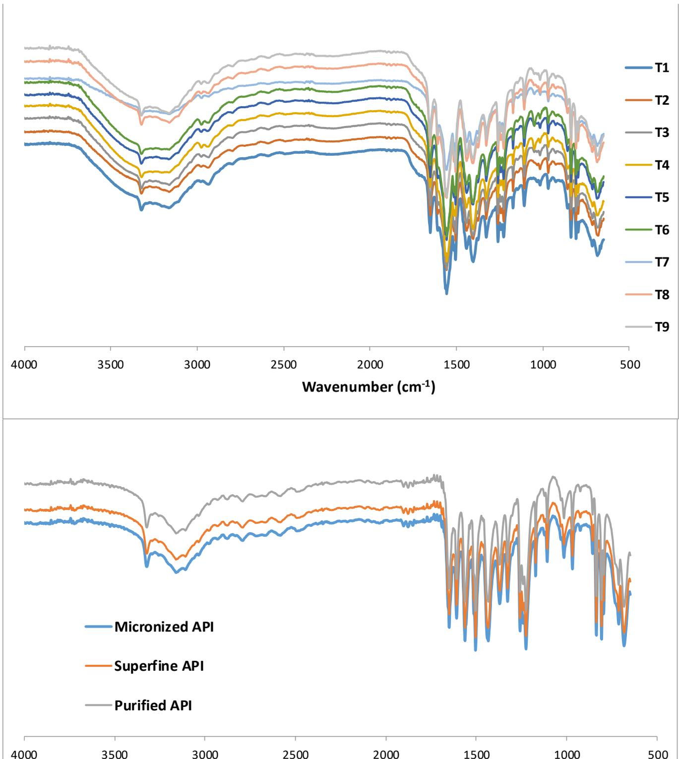
**Figure 3:** FT-IR analyses of matrix types of tablets and Paracetamol's APIs.
