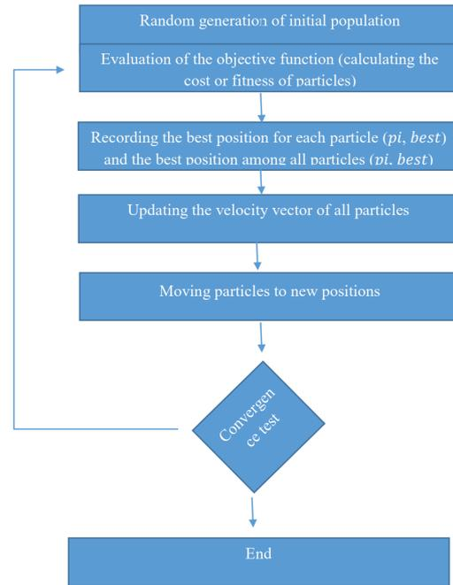
**Figure 3.** Graphical Representation of the Particle Swarm Optimization Process for Optimizing the Number of Neurons in Hidden Layers Within Neural Network Architectures.
