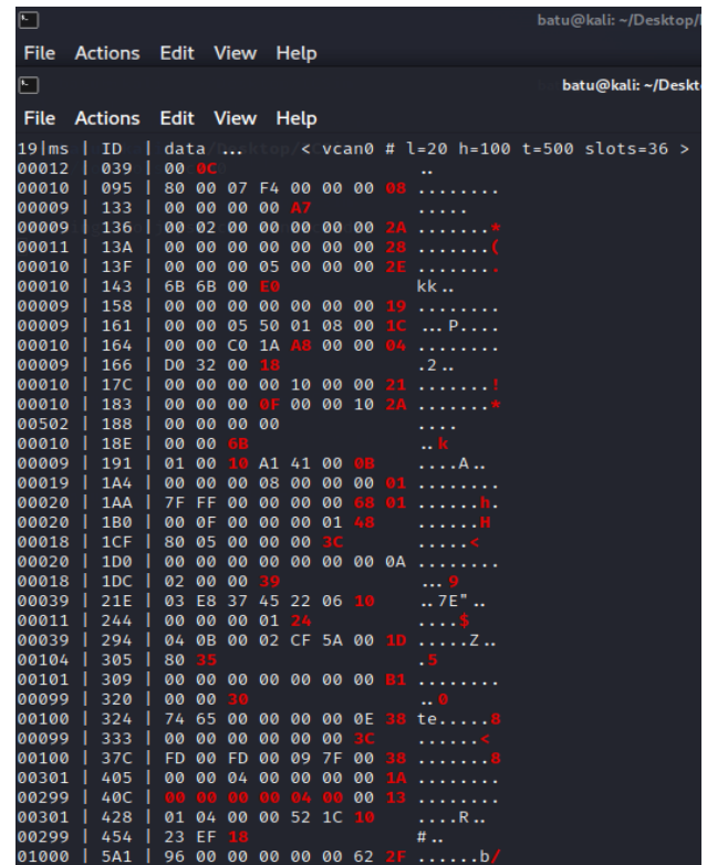
Figure 5. CAN network packets captured on ICSim
