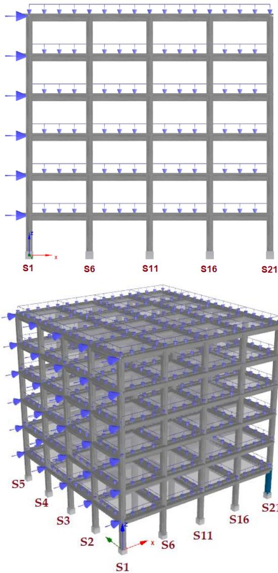
Figure 7. 2D and 3D structural models and representation of some columns
