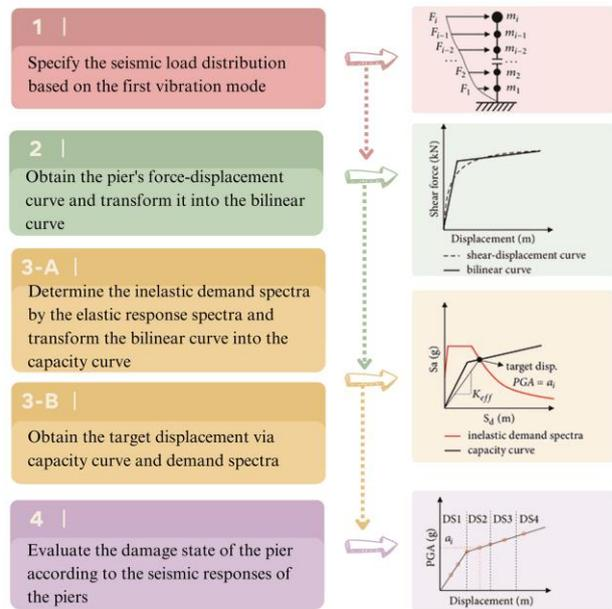
Figure 5. Flowchart of pushover analysis modified from Guo et al. [61]
