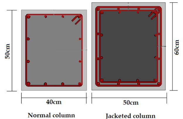
Figure 8. Column cross-sections before and after jacking
