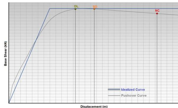
**Figure 12.** Typical pushover and idealized capacity curves
