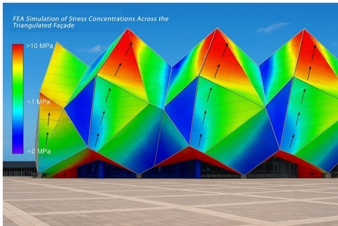
Figure 12. FEA simulation illustrating stress concentrations across the triangulated façade of Baku Crystal Hall. Red zones indicate areas of high stress; blue zones show lower load impact. Modeled for representational purposes using Rhino + Karamba3D by author, 2025. (Adapted from principles in Tam et al., 2022; Kolarevic, 2003).
