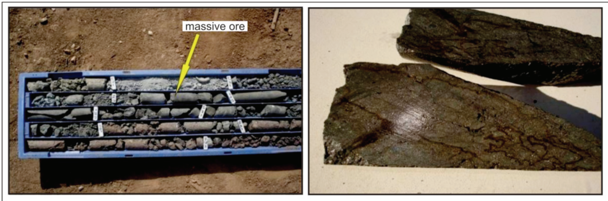
Figure 10- Massive ore mineral cut in drilling AS -2 and close up view from this bisected ore
