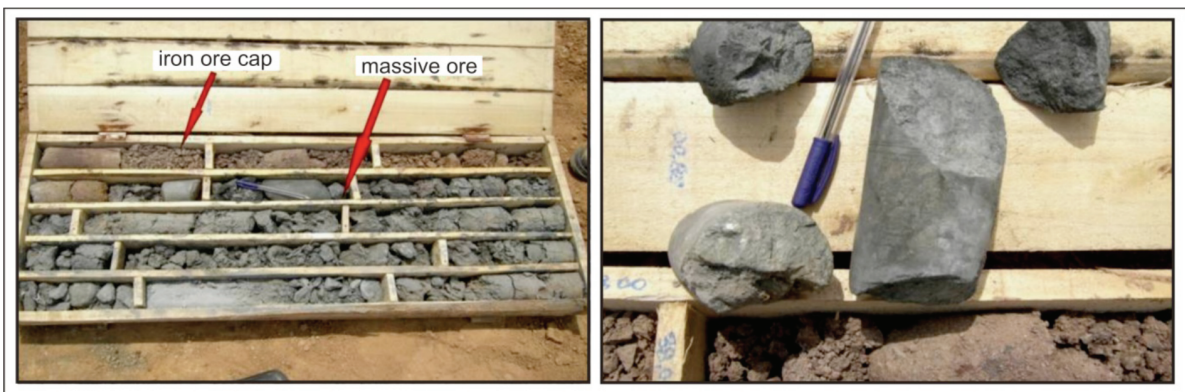
Figure 11- Iron ore cap (gossan) that was cut in drilling AS-9 and view from cataclastic massive ore minerals in patches
