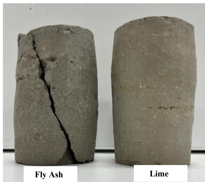
Figure 10. Different failure modes for stabilized soil samples.
