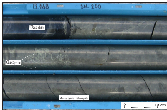
Figure 16- Chalcopyrite veins within massive pyrite, chalcopyrite in Mağaradoruk deposit.
