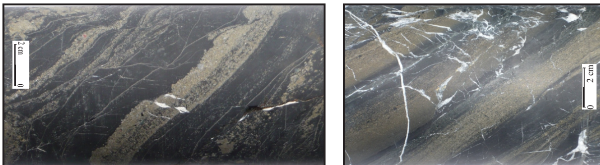
Figure 11- Traces of sorting in massive ore bands which are formed by pyrite and chalcopyrite in black shale.
