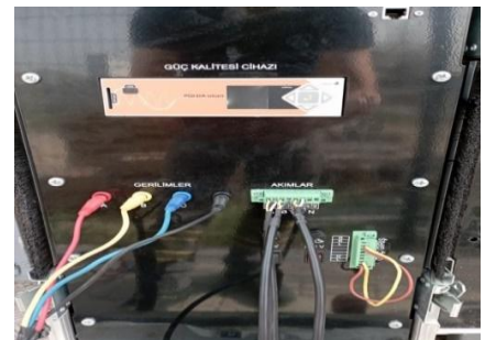
Figure 2. Power quality measurement device with A-Eberle energy analyser
