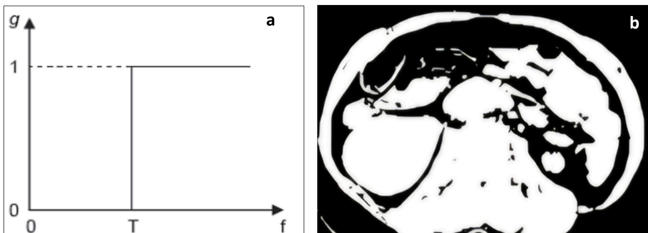
Figure 3. Thresholding Step: (a) Single value threshold and graphical representation of the threshold for a specified value; (b) Results obtained from the thresholding process in MATLAB.
