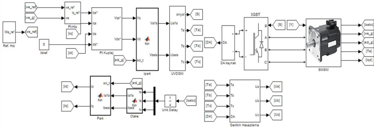
Fig. 3 Field oriented control Simulink overall blocks
