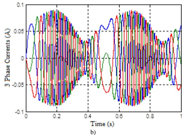
The figures of the field oriented control of the PMSM made at variable input speed reference values are given below. In the following, the speed change of the sinusoidal wave from 1000 rpm to -1000 rpm is investigated, then the speed change of the square wave from 1000 rpm to -1000 rpm, and the speed change of the triangle wave from 1000 rpm to -1000 rpm were investigated.
