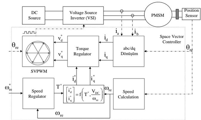
Fig.2. Field oriented control design
