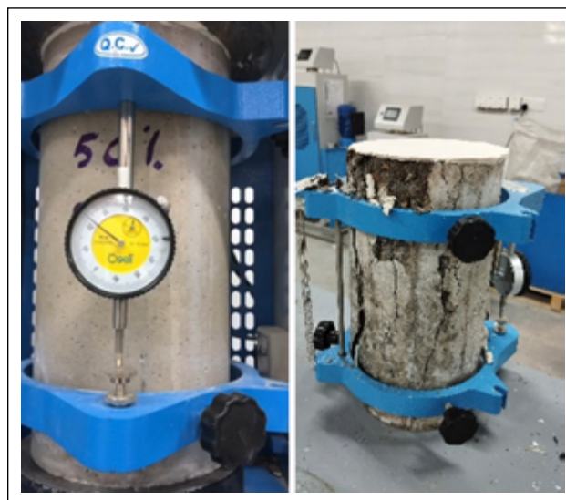
Figure 5. Measuring the stress-strain curve (left image is before testing, right image is after testing).
