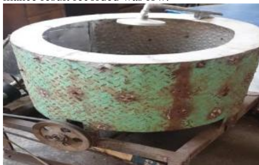
Figure 17. Cassava peeler powered by 1hp
