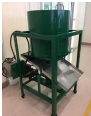
Figure 12. Electrical motor driven cassava slicer.
