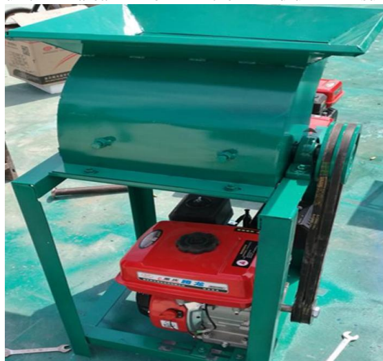
Figure 6. Electric motor driven cassava grater
