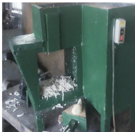
Figure 11. Reciprocating type cassava slicing machine
