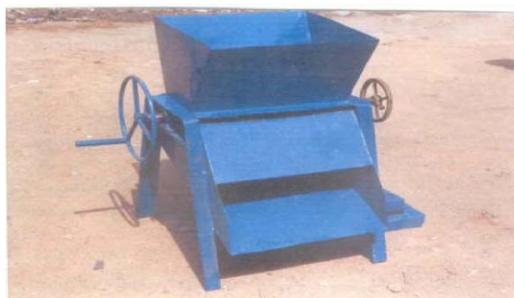
Figure 4. Dual-operation cassava grater.
