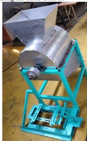
Figure 8. Diesel engine-operated cassava grater
