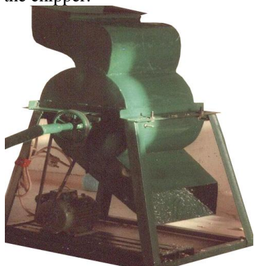
Figure 16. Electric motor cum manually operated chipper
