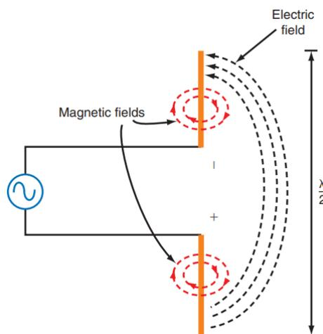
*Figure 1. The electric and magnetic fields around the transmission line*
