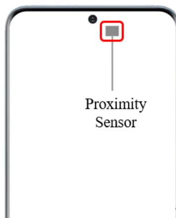
**Figure 4.** Enable Proximity Sensor by moving phone to the ear
