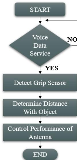
*Figure 5. Flow diagram of controlling antenna performance by using a grip sensor*
