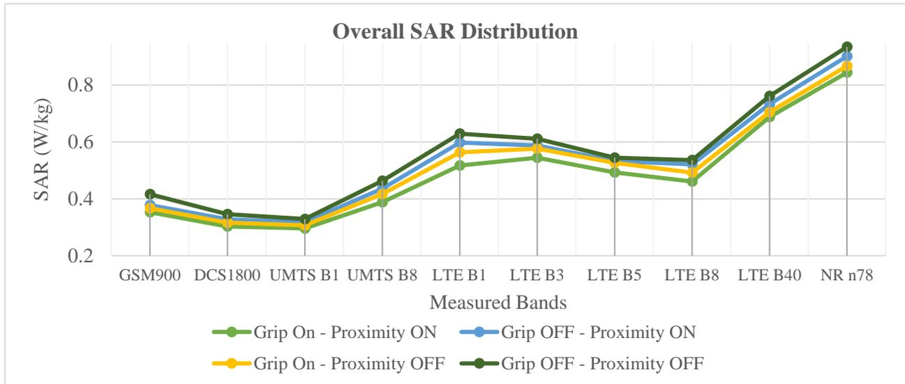
**Figure 7.** Overall SAR measurement results, for 2G, UMTS, LTE and 5G NR
