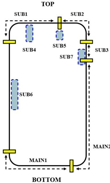
Figure 6. Rear (Back side) view of DUT, illustrate antenna placements
