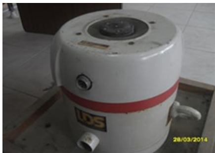
Figure 2. LDS V450V electromagnetic shaker with 311 N sinus load capacity
