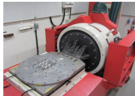
Figure 1. Electrodynamic shaker, direction changing system and slip table system [12]
