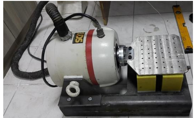
Figure 16. Assembly of slip table, connection parts shakers
