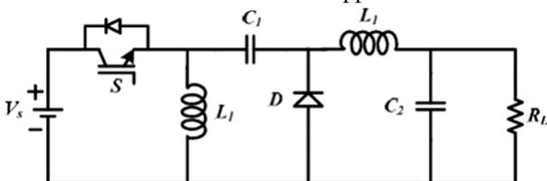
Figure 1. Zeta DC-DC Converter
