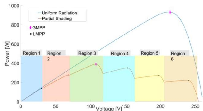
Figure 2. P-V graph resulting from uniform radiation and PSC in the PV system.
