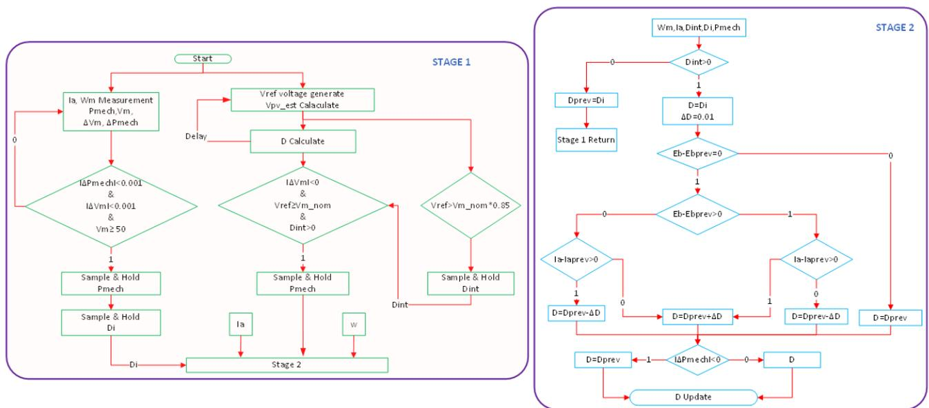
Figure 3. Flow chart of the proposed MPPT algorithm.
