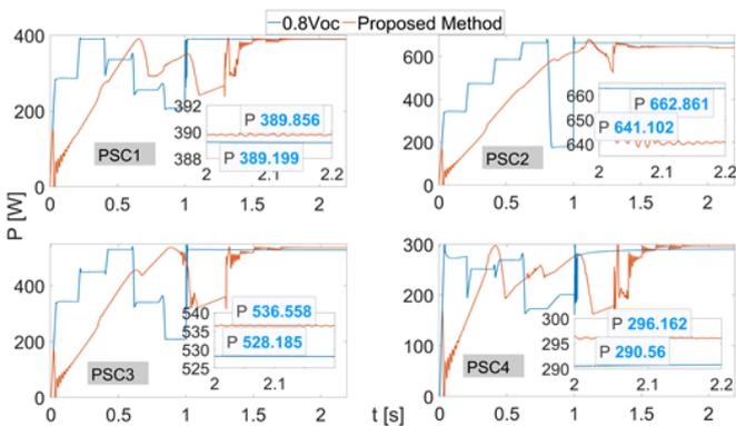
Figure 6. Power obtained using 0.8Voc and proposed MPPT methods in four different PSC
