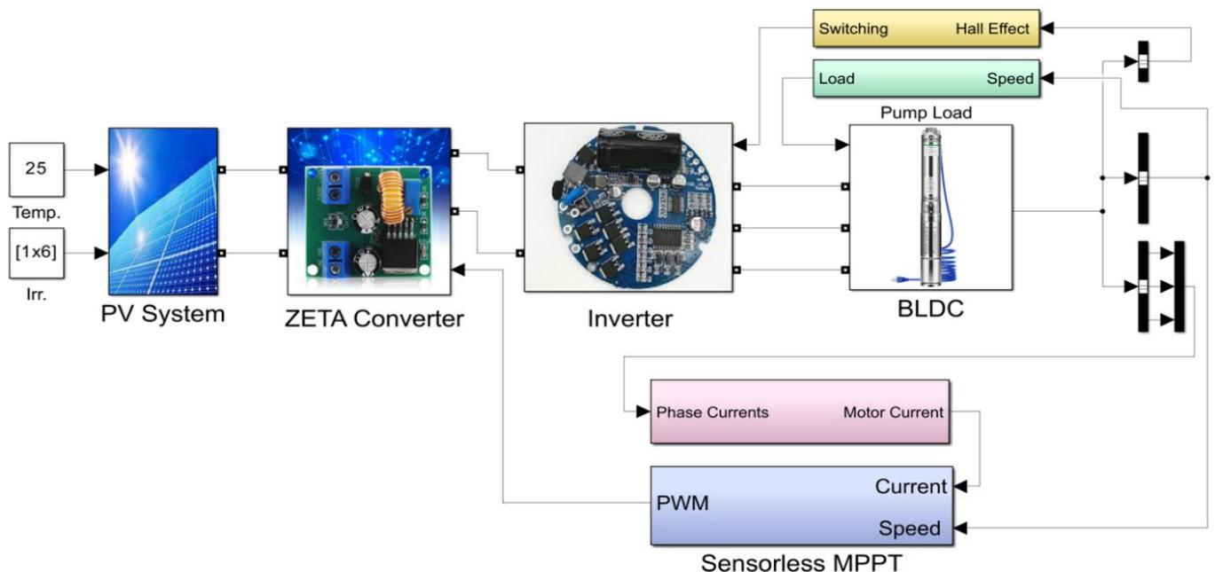
Figure 4. MATLAB/Simulink simulation of the PV pump system
