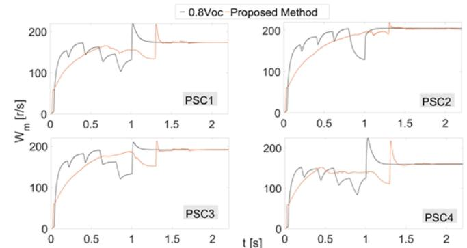
Figure 8. Speed of the BLDC motor obtained with 0.8Voc and proposed MPPT methods
