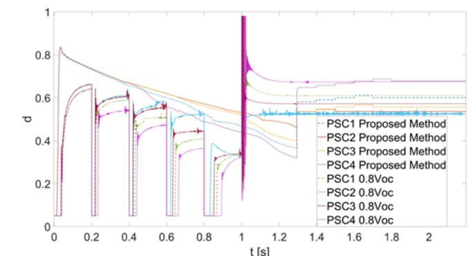
Figure 9. Duty periods obtained with 0.8Voc and proposed MPPT methods
