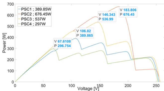
Figure 5. Maximum powers obtained from PV systems operating under four different PSCs
