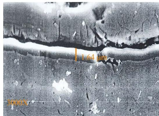
**Figure 4.** SEM cross-section of TiN coating deposited at 100 V bias voltage, indicating the measured coating thickness (1.64  $\mu\text{m}$ ) and its interface with the substrate
