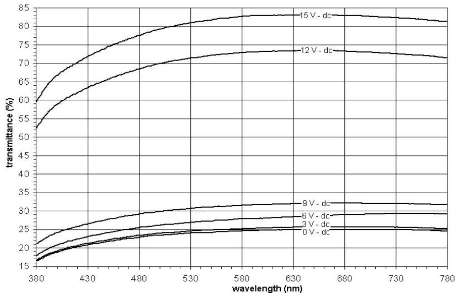
**Figure 2.** Transmitted intensity versus wavelength under different DC voltages.
