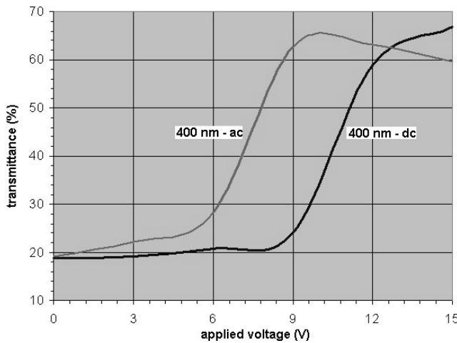
**Figure 4.** Transmitted intensity versus applied voltage at 400 nm for AC and DC voltages
