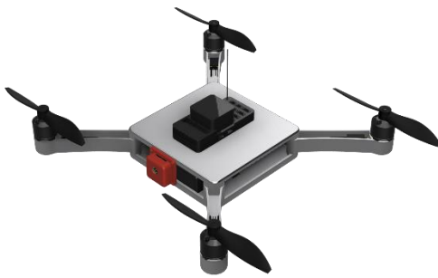
Fig. 2. Assembly model of quadcopter structure type drone
