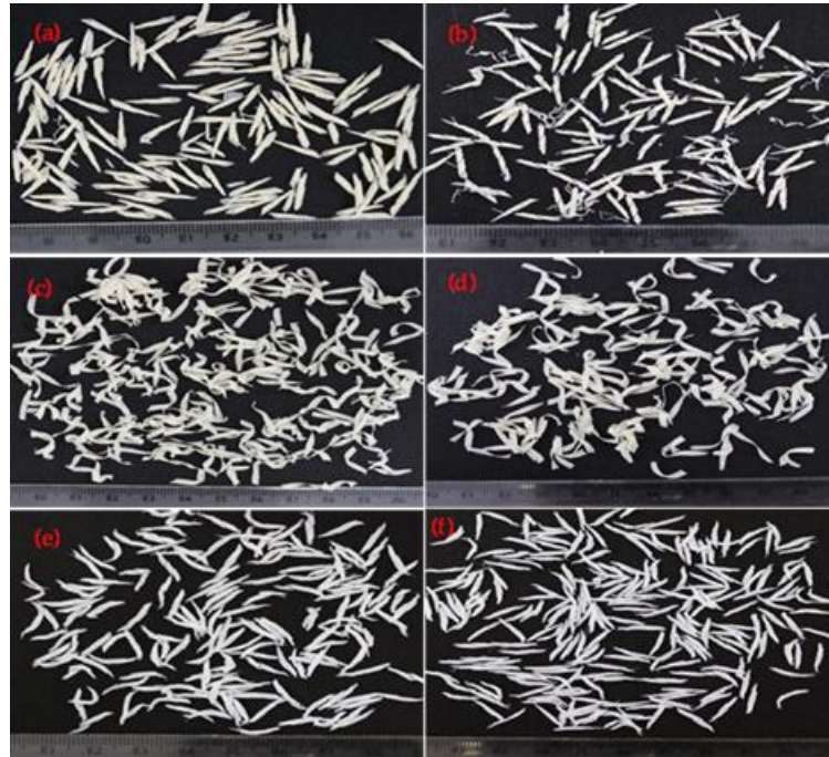
Figure 7. Chip forms: (a) without heat treatment-PEEK, (b) with heat treatment-PEEK (c) without heat treatment-PP (d) with heat treatment-PP, (e) without heat treatment-PTFE and (f) with heat treatment-PTFE
