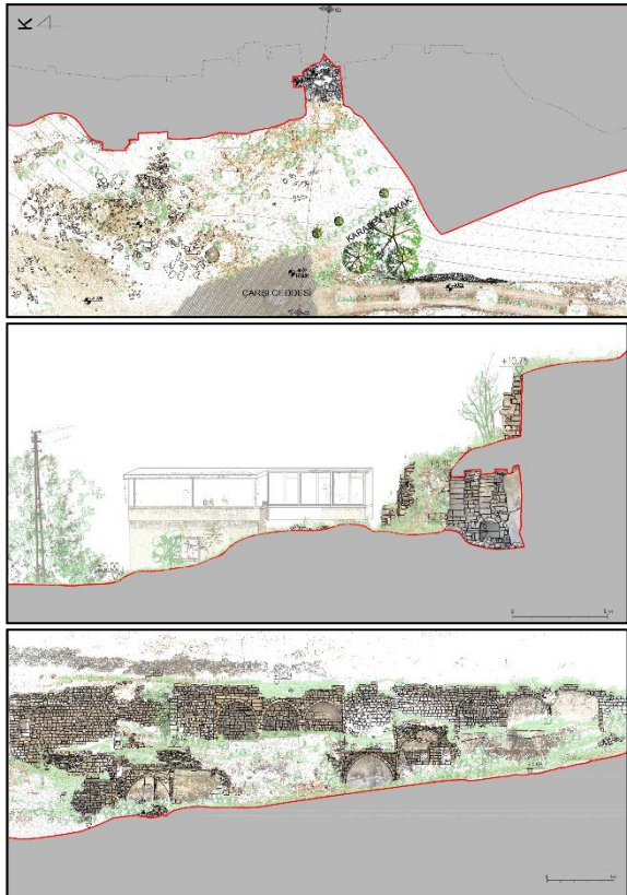
Figure 17. Arched Building +1.660 Elevation Plan, A-A Section and Façade Orthophoto [25]
