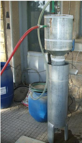
Figure 3. a picture of the experimental device UASB
