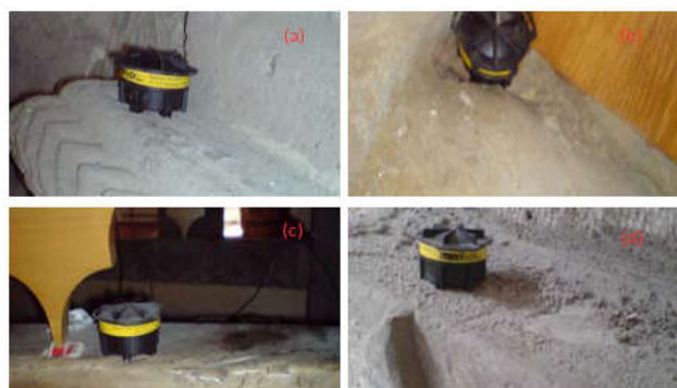
Figure 1. Photograph of located one-piece of a CR-39 detector cup in the Sungur Bey mosque (a), the Alaeddin mosque (b), the Disari (Celebi Husamettin) mosque (c) and in the Ak Medrese Culture House (d) here in Nigde.
