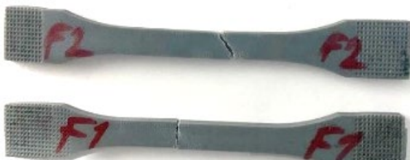
Figure 1. Tensile test specimens are made up of Tough-PLA (after the tensile test)
