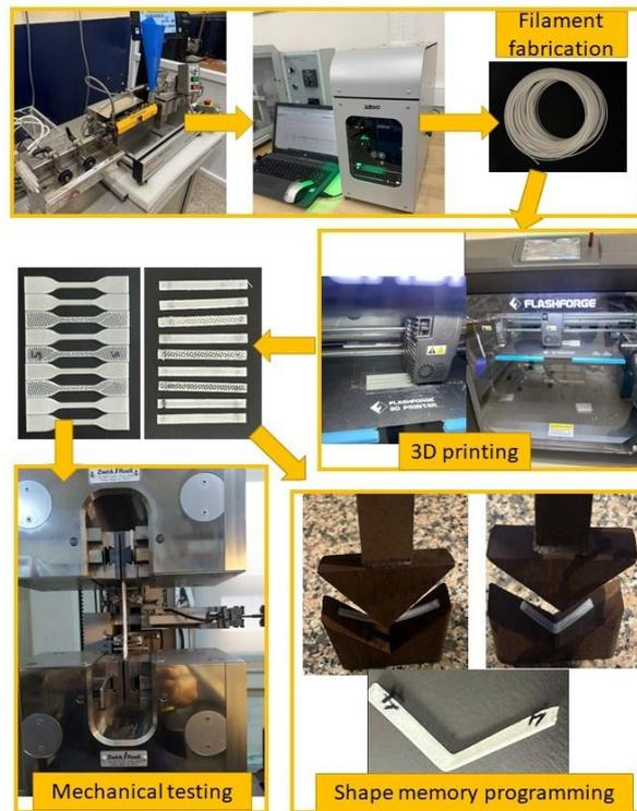
**Figure 4.** Experimental setup and workflow of the study
