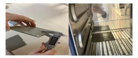
**Figure 4.** Application of 0.2 mm thick mask on glass plate and determination of drying time (37 °C-oven, n=3)
