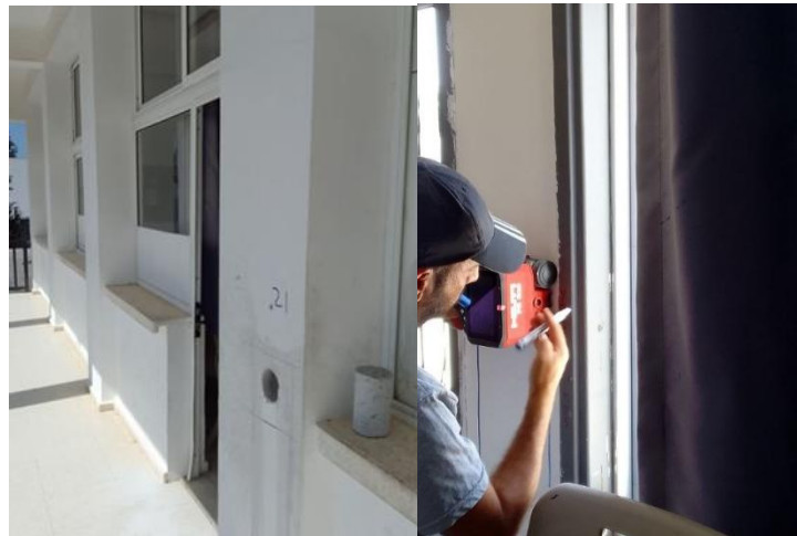
Figure 4. Laboratory test for validation; a) Extracted concrete cores for compression test; b) Scanning concrete rebars
