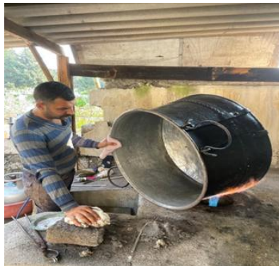
Image 13: Heating the Copper Cauldron
