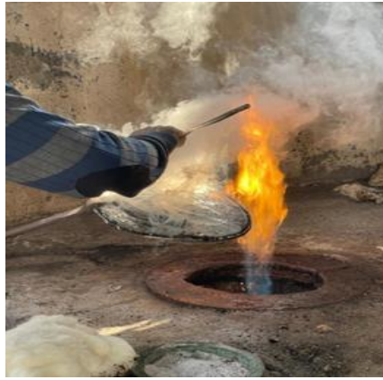
Image 15: Applying the Tin Rod to the Product
