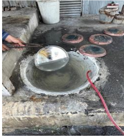
Image 10: Process of Immersing the Copper Tray in the Cooling Pool
