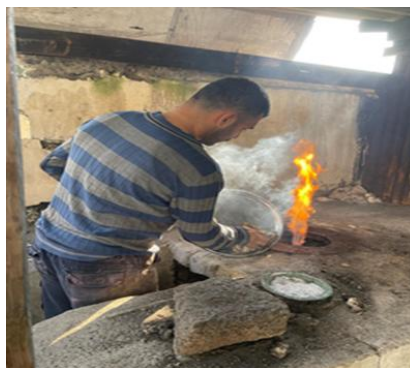
Image 14: Sprinkling Ammonium Chloride on the Copper Tray
