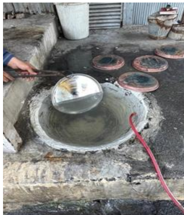
Image 16: Cooling the Tinned Tray
