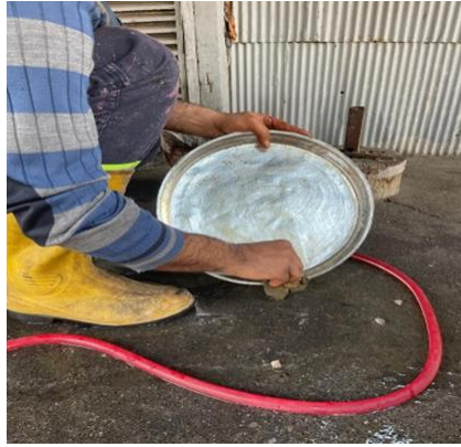
Image 12: Copper Tray Washed with Sand
