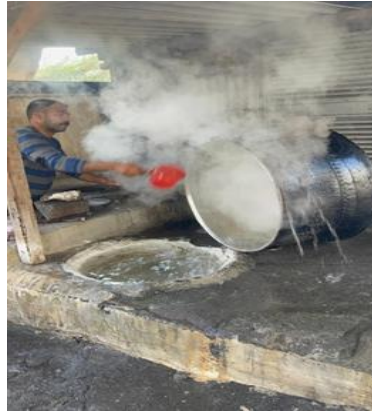
Image 17: Cooling the Tinned Cauldron
