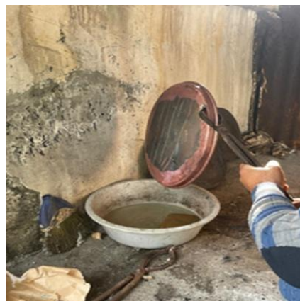
Image 11: Copper Tray Cleaned with Caustic
