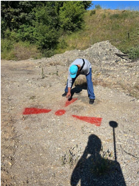
Figure 3. Installation of a GCP
