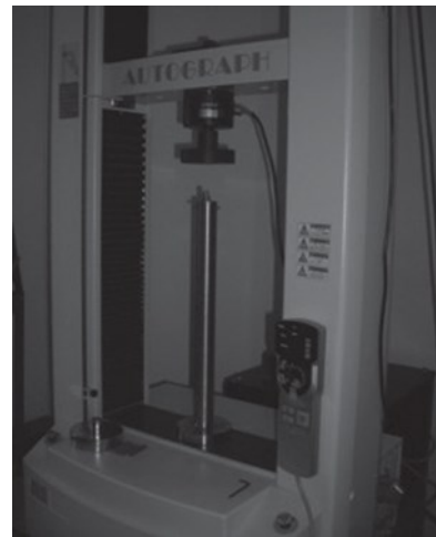
Figure 2 : Photography of the 3-point bending test of proximal tibia locking screws.
