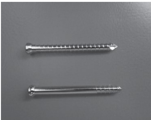
Figure 1 : Samples of proximal tibia locking screws (Above:Low threaded, Below: Unthreaded).
