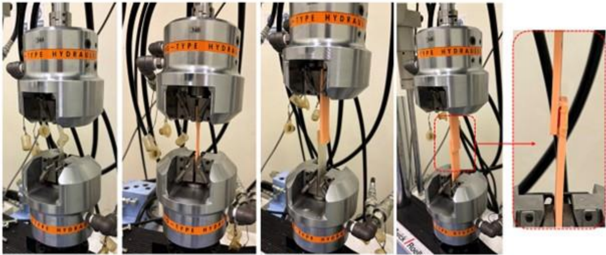
Figure 7. The tensile testing process for tensile and adhesive specimens
