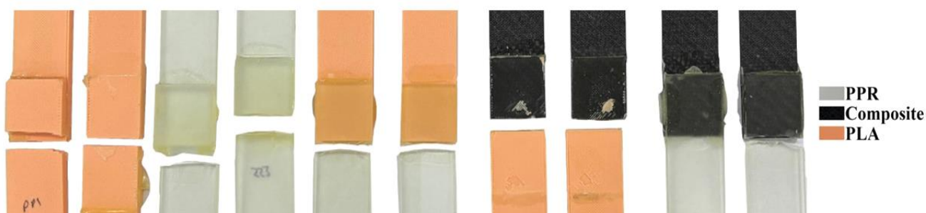
Figure 10. Failure surfaces of the SLJ adhesive specimens
