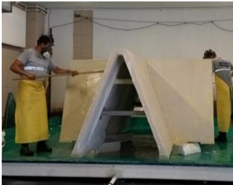
Figure 7. Application of the acid solution to the GFRC panel surface
