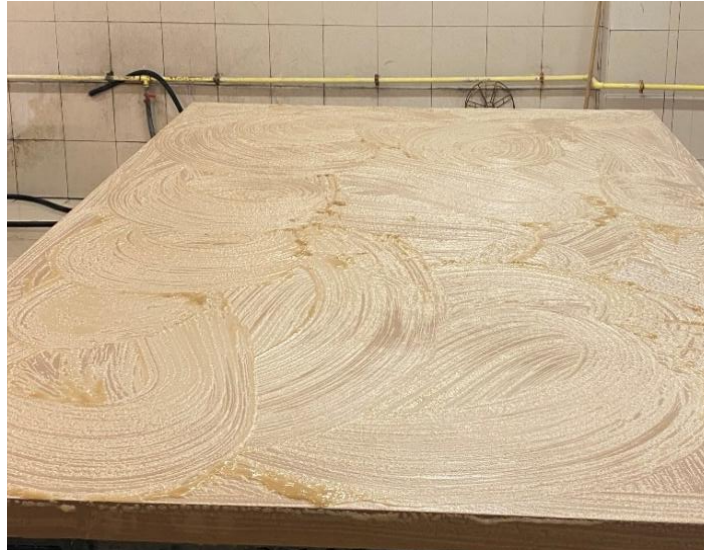
Figure 8. Keeping the solution on the GFRP panel surface
