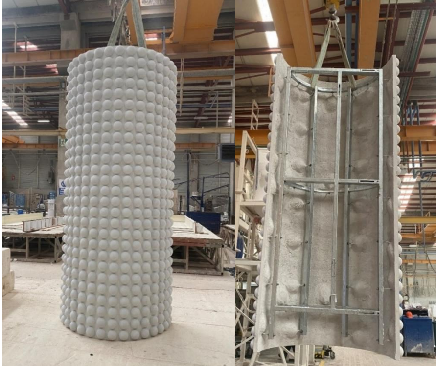
Figure 6. Front and back sides of the GFRC panel
