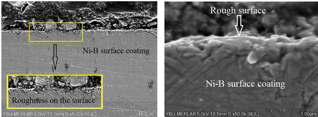
Figure 10. Ni-B coating cross sections at different magnifications [17, 18].
