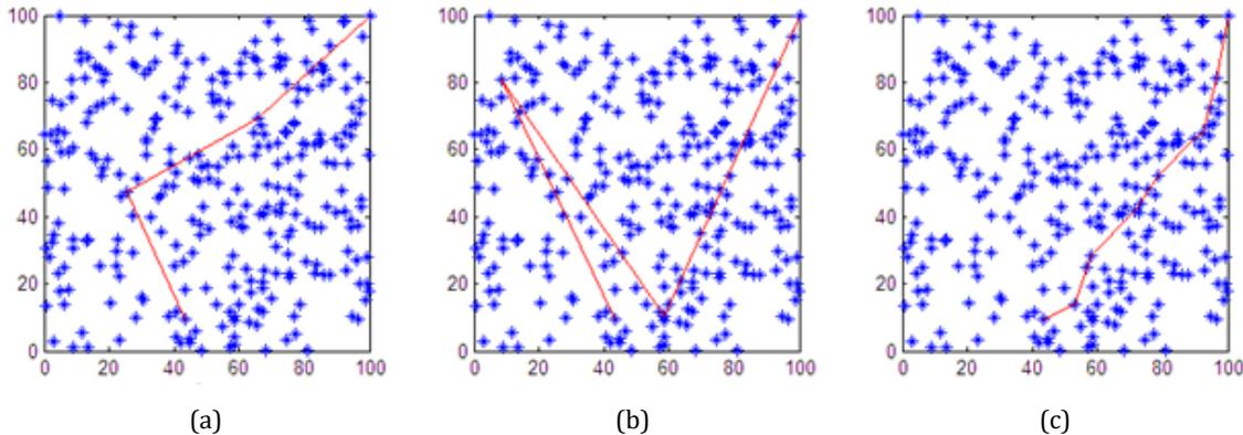
**Figure 7.** Routing operation for random event 3 detection (a) Routing based on the error parameter, b) Routing based on error and energy parameters, c) Routing based on error, energy and distance parameters (optimal path)).
