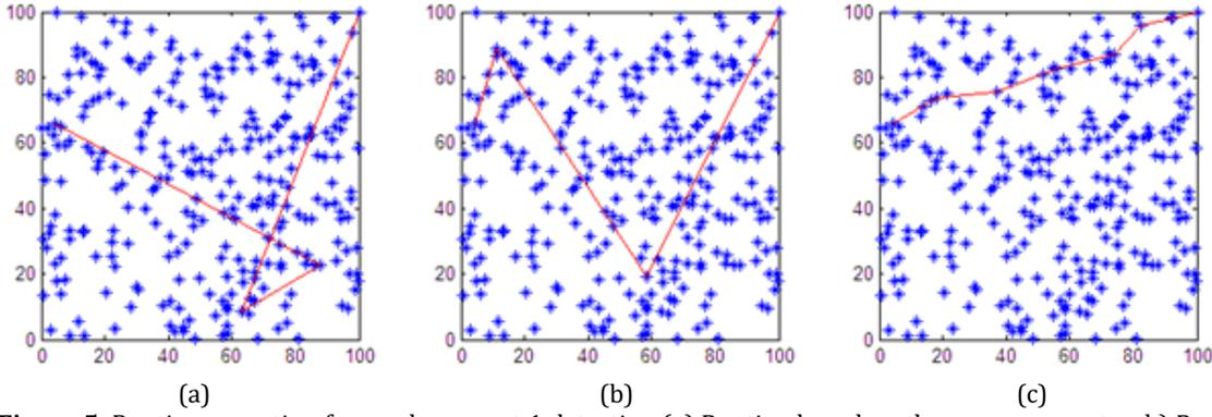
**Figure 5.** Routing operation for random event 1 detection (a) Routing based on the error parameter, b) Routing based on error and energy parameters, c) Routing based on error, energy and distance parameters (optimal path)).
