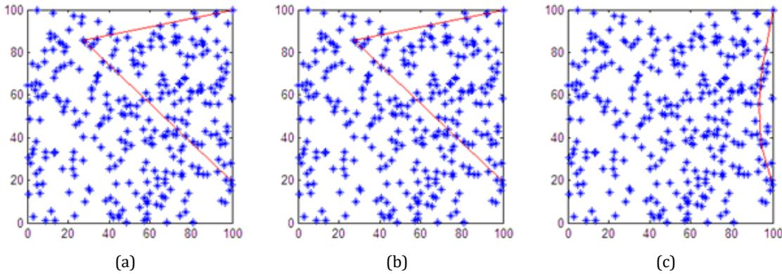
**Figure 6.** Routing operation for random event 2 detection (a) Routing based on the error parameter, b) Routing based on error and energy parameters, c) Routing based on error, energy and distance parameters (optimal path)).
