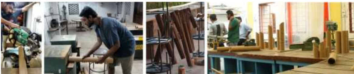
Fig. 2. Hands on work with paper-tube: cutting, grinding and waterproofing
