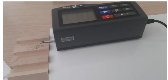
Figure 7. Roughness measurement of specimens
