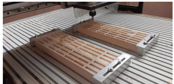
Figure 6. CNC machining of specimens
