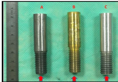
Figure 3. The other three BB, Stainless-steel (A), Brass (B), Aluminum C, red arrow is showing the hole that is for placing the first thermocouple.
